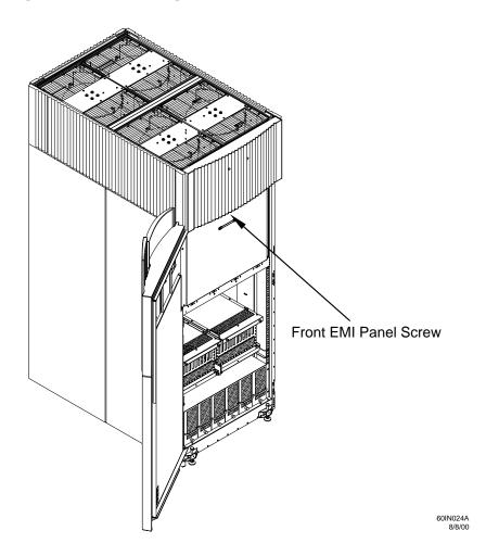
**Step 2.** Use the handle provided to remove the EMI panel and set it aside.
