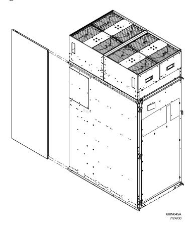
**Step 3.** Attach the skin *without the lap joint* (front) over the top bracket and under the bottom bracket and gently slide the skin into position.
