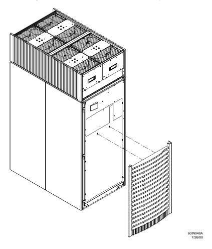
**Step 4.** Using a Torx 10 driver, secure the lower door bezel to the front door chassis with 10 of the screws provided (HP P/N 0515-0372). Insert all screws loosely, then torque them after the bezel is aligned.
