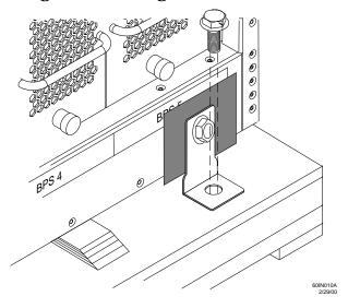
**Step 6.** On the other side of the pallet, remove only the bolt on each mounting bracket that is attached to the SPU cabinet.
