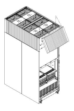
**Step 3.** Align the bezel over the nuts that are attached to the bracket at the front of the cabinet.
