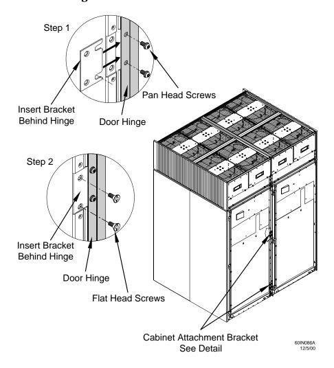
**Step 3.** Attach the remaining four (4) flathead screws (0515-3210) provided to install the brackets to Cabinet 0, two for each bracket.
