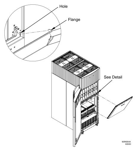
2. Position the panel at the top lip and lift the panel up while pushing the bottom into position. You may have to compress the EMI gasket to get the panel to seat properly.
