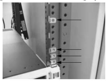
**Step 3.** Install the Tape Array 5300 rack shelves into the rack using the supplied procedure.
