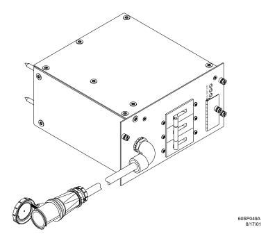
Figure 3-15 Four-Wire Connector
