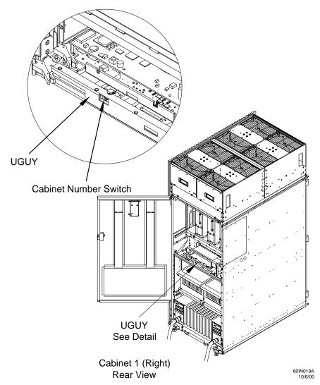
If the switch is not set to **1**, change it by turning the thumbscrew.
