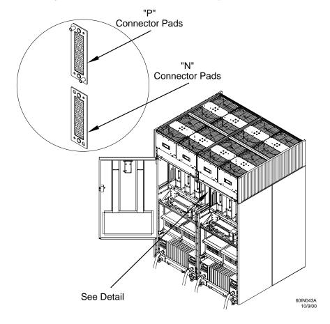
**Step 1.** Install the six 5-inch cables between the two cabinets.
