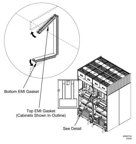
**Step 3.** Attach the top access panel EMI gasket.
