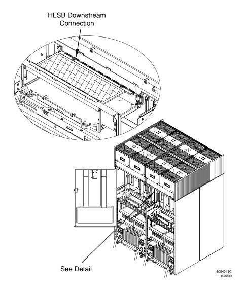
The following figure shows what the Upstream and Downstream connections look like after they are installed.
