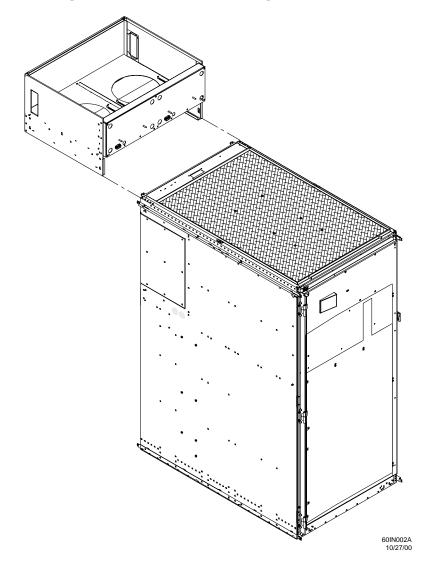
Unpacking and Installing the Blower Housings and Blowers
