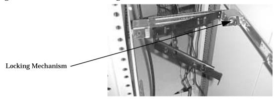
Once mounted, the TFT5600 may be pulled out on its slides. The slides lock whenever the unit is pulled out.
