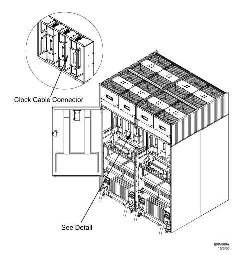
2. Uncoil the clock cable and connect it to the RBP connector on the Cabinet 0 UGUY board.
