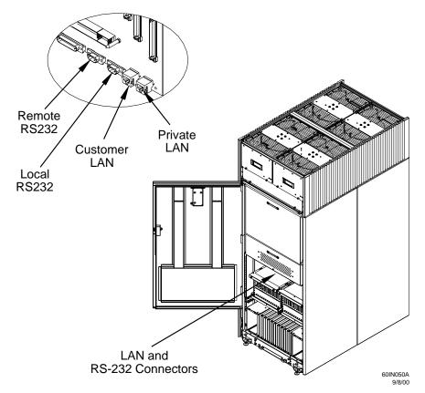
**Step 2.** Connect the other end of the RS-232 cable to the CE tool.
