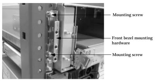
**Step 7.** Attach the Tape Array 5300 front bezel.
