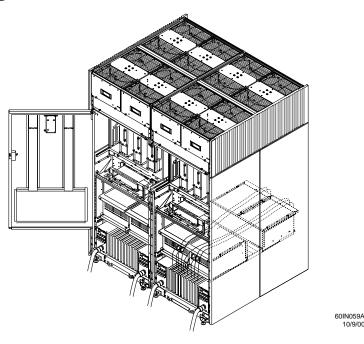
Use the following procedure and guidelines to route cables through the cable groomer at the bottom rear of the cabinet.
