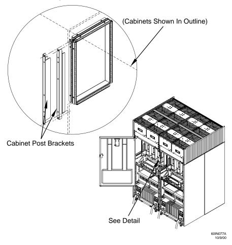
**Step 6.** Install the latch catch that was removed from the cable access panel to the cabinet post bracket.
