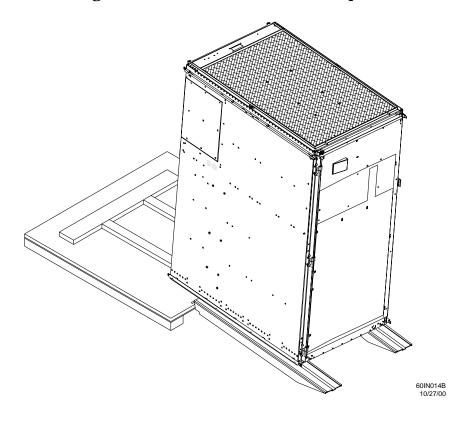
WARNING Do not attempt to move the Superdome cabinet, either packed or unpacked, up or down an incline of more than 15°.
