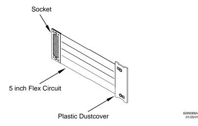
**Step 7.** Install the flex cables.
