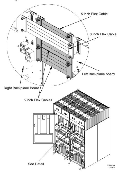
**Step 3.** Inspect the cables to verify that they are installed properly.
