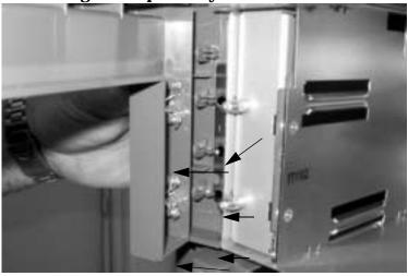
**Step 8.** Install the drive bay bezels for vacant drive bays slots.
