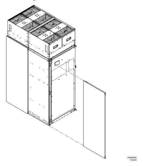
**Step 4.** Push the side skins together, making sure the skins overlap at the lap joint.
