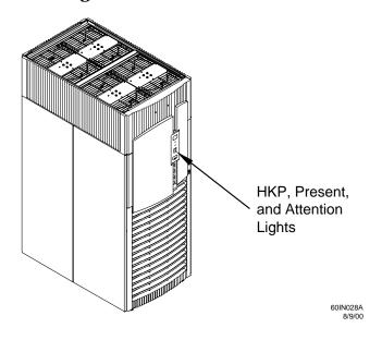
**Step 2.** Check the Bulk Power Supply (BPS) LEDs.
