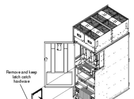
Figure G-6Cable Access Panel (after removal)
