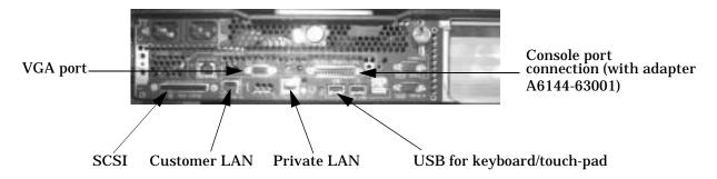
**Figure A-16 SMS Connections**
