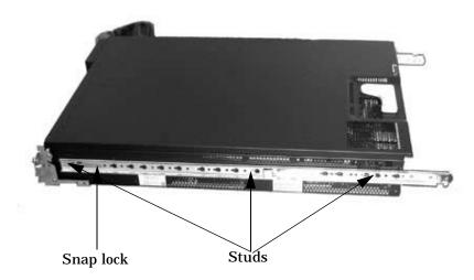
**Step 4.** Using two people, carefully lift and align the equipment slides on the hp Server rx2600 to the equipment slides in the rack.
