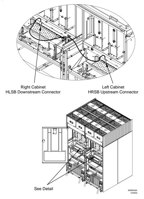
$\textbf{Step} \quad \textbf{3.} \ \, \textbf{Inspect all flex cables for damage before installing them}.$
