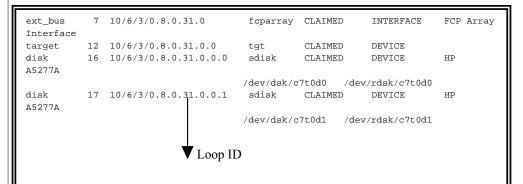
Protocol Type is 8 (8 = mass storage) Area is 0 in private loop Port is equivalent to loop ID BUS (0-7) Target (0-15) LUN (0-7)
