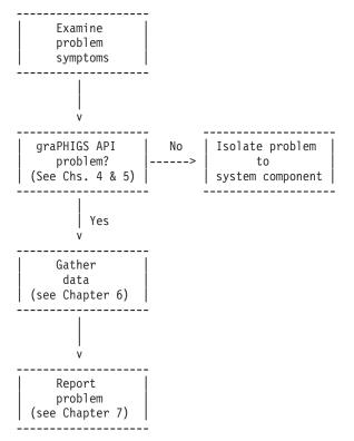
This chapter contains the basic procedures used to identify problems in the hardware and operating systems that the graPHIGS API uses. First, examine the following areas to determine whether they function properly. Programs using the graPHIGS API can fail because of problems with any of the following:
