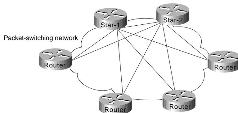
There are many forms of partially meshed topologies. In general, partially meshed approaches are considered to provide the best balance for regional topologies in terms of the number of virtual circuits, redundancy, and performance.
