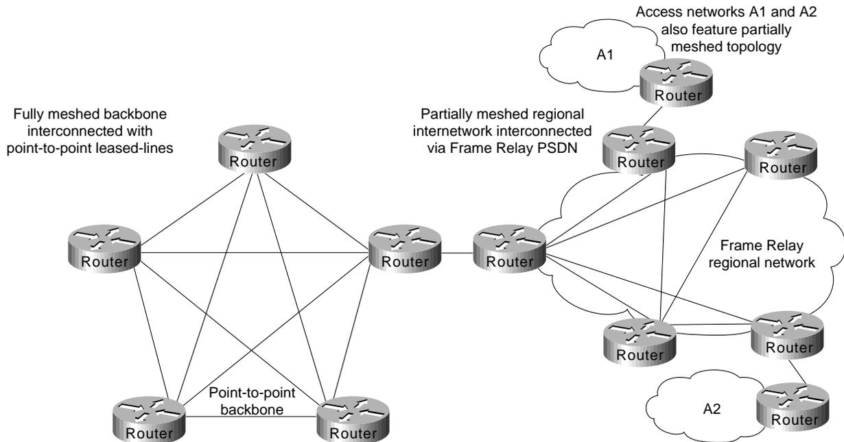
Hybrid hierarchical meshes have the advantages of providing higher performance on the backbone, localizing traffic, and simplifying scaling of the internetwork. In addition, hybrid meshed internetworks for Frame Relay are attractive because they can provide better traffic control in the backbone and they allow the backbone to be made of dedicated links, resulting in greater stability.
