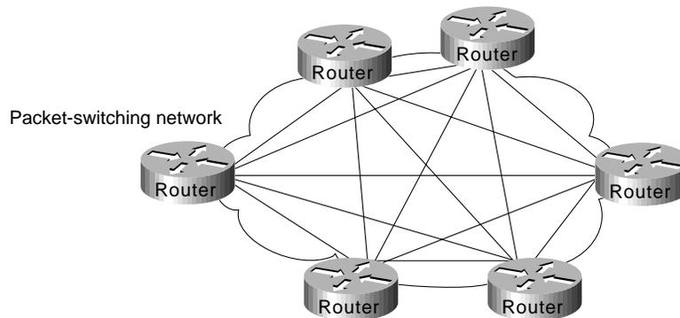
The key rationale for creating a fully meshed environment is to provide a high level of redundancy. Although a fully meshed topology facilitates support of all network protocols, it is not tenable in large packet-switched internetworks. Key issues are the large number of virtual circuits required
