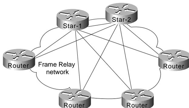
A feature called *virtual interfaces* (introduced with Software Release 9.21) allows you to create internetworks using partially meshed Frame Relay designs, as shown in Figure 9-8.
