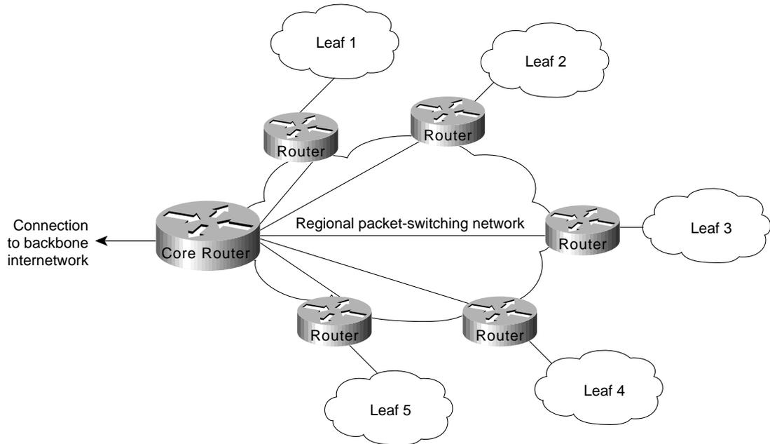
The advantages of a star approach are simplified management and minimized tariff costs. However, the disadvantages are significant. First, the core router represents a single point of failure. Second, the core router limits overall performance for access to backbone resources because it is a single pipe through which all traffic intended for the backbone (or for the other regional routers) must pass. Third, this topology is not scalable.
