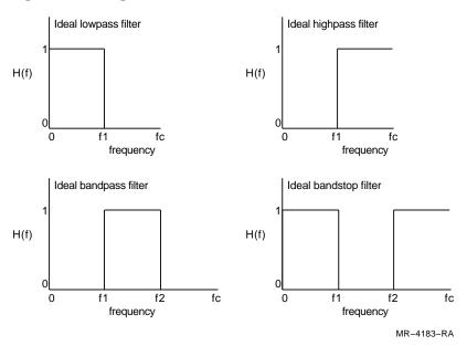
In Figure 11-1 fc refers to the Nyquist frequency  $1/(2\Delta t)$ ,  $\Delta t$  is the time between data samples, and f1 and f2 refer to the frequency values where filtering is to be applied.
