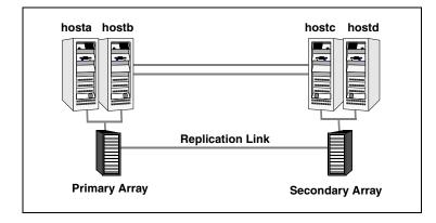
Two hosts (hosta and hostb) are attached to the primary array, and the other hosts are attached to the secondary array. The application is running on hosta and devices in the local array are P-VOLs in the PAIR state.
