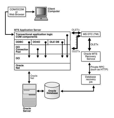
Figure 5–1 Component Integration in a Transaction
