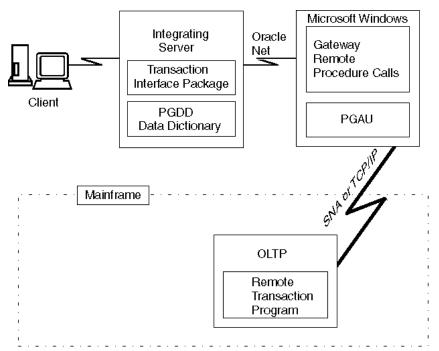
Figure 1–1 provides an illustration of the relationship between the gateway and the Oracle Integrating Server on a Windows host. The client is connected to the Oracle Integrating Server, which is connected to the gateway, which holds the gateway remote procedure calls and PGAU, via Oracle Net . They are connected to the OLTP in the Mainframe via TCP/IP or SNA. Figure 1–1 is adequately described in the text surrounding it.
