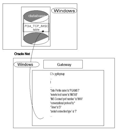
Figure 6–1 illustrates how the pg4tcpmap tool maps the Side Profile Name to TCP/IP and IMS Connect attributes from the gateway into the PGA\_TCP\_IMSC table. The process of mapping information to TCP/IP is described in the surrounding text.
