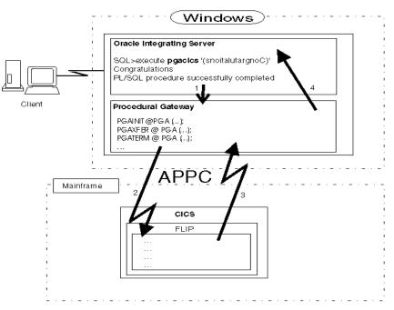
Figure 1–3 Communication Between the Oracle Server and the Mainframe, Using SNA
