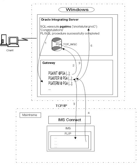
Figure 1–4 illustrates the communication flow between the gateway and the mainframe, when using the TCP/IP communication protocol. This figure is adequately described in the section preceding it.
