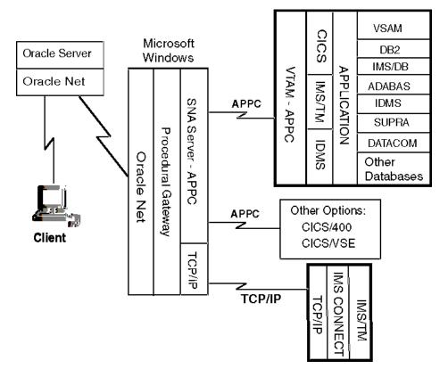
Figure 1–2 Gateway Architecture Featuring SNA or TCP/IP Protocol
