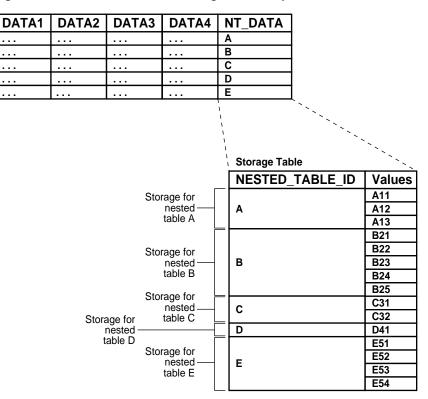
Figure 8–4 Nested Table in IOT Storage with Compression
