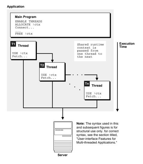
Figure 12–1 Loosely Coupling Connections and Threads
