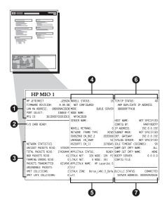
Figure 6.2 Ethernet Configuration Page (Internal MIO Print Servers)
