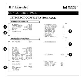
Figure 6.5 Token Ring Configuration Page (Internal EIO Print Servers)
