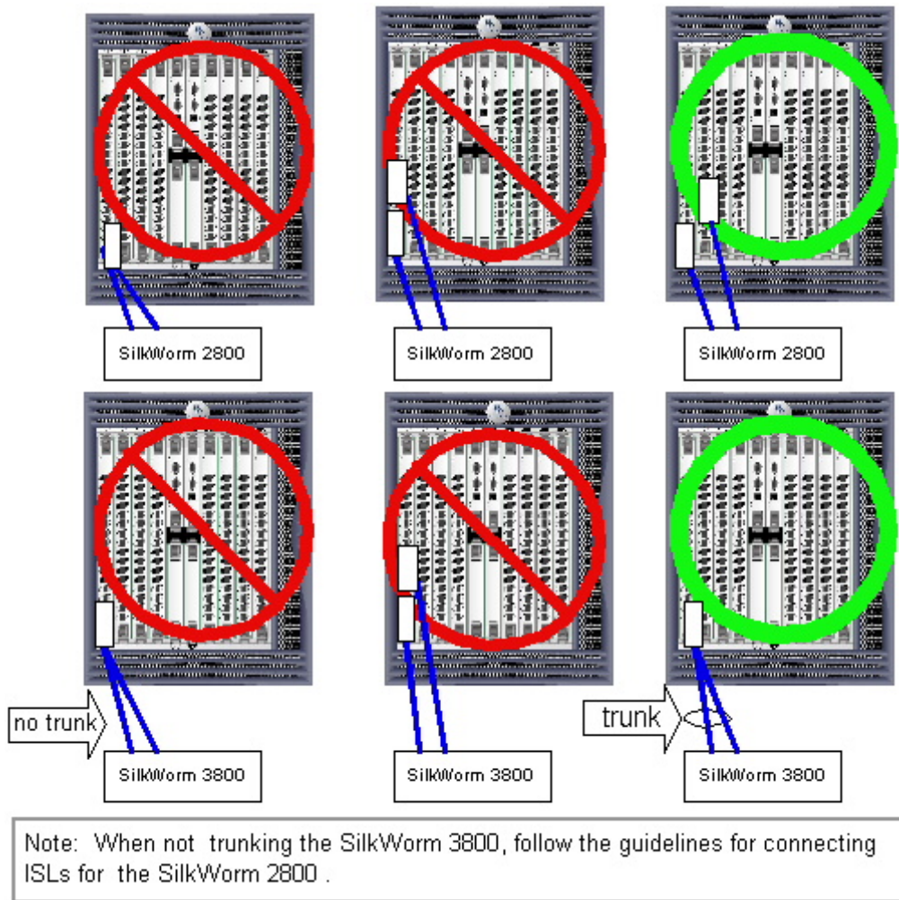
Figure 2-13 Do not connect more than one ISL to the same switch port card unless it is part of a trunk.
