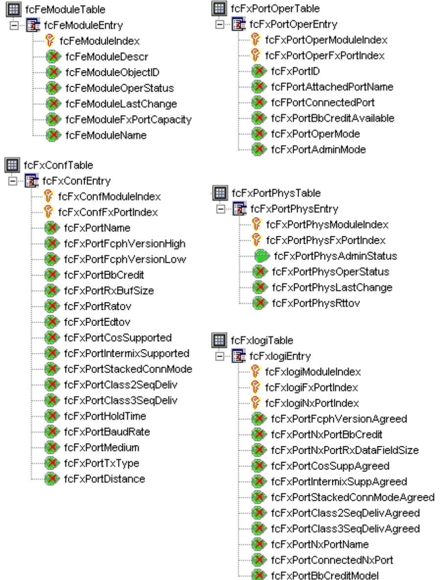
Figure 9. Tree Structure for fcFeConfig and fcFeOpTables
