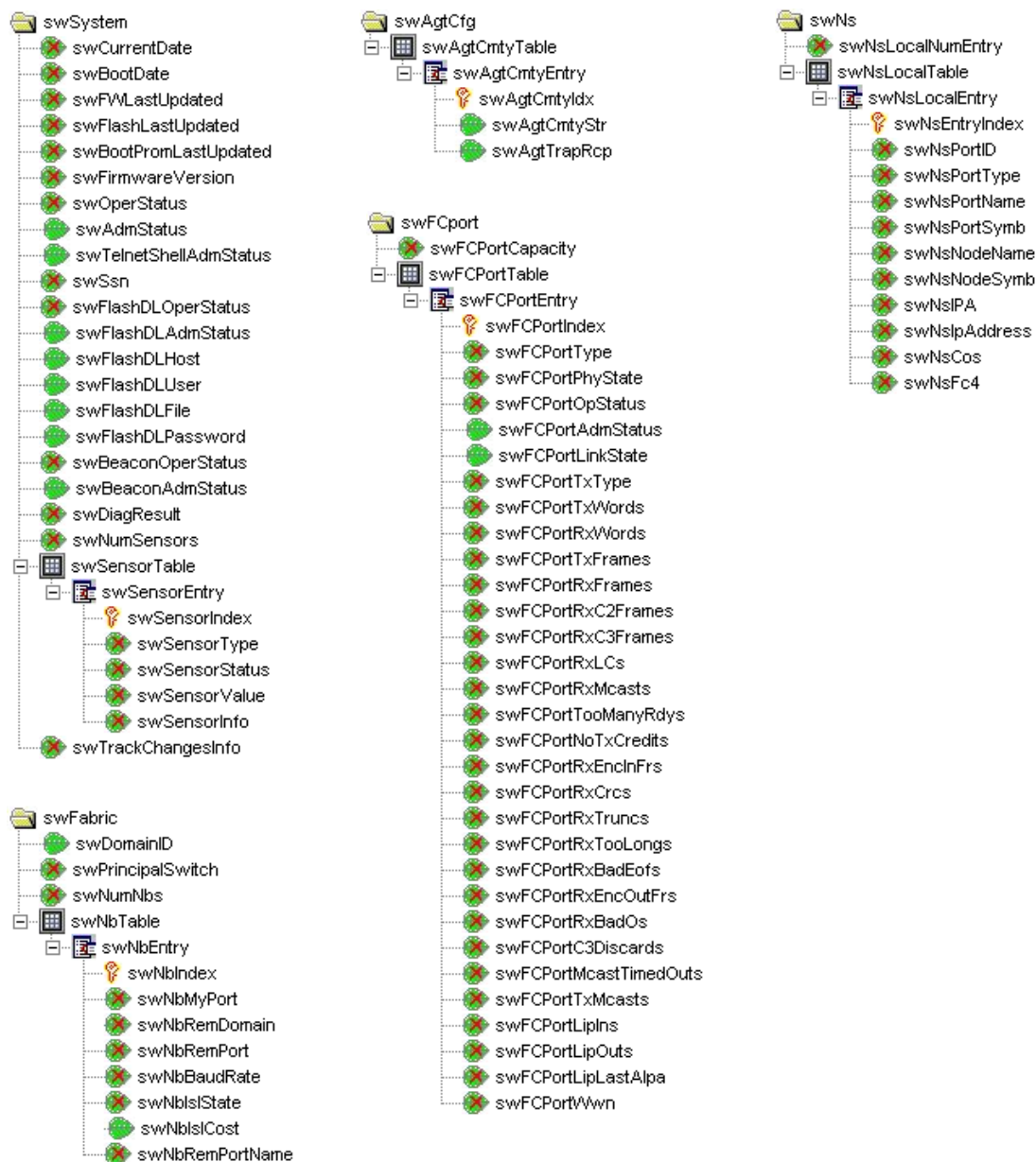
Figure 12. Tree Structure for swSystem, swFabric, swAgtCfg, swFCPort, and swNs Groups
