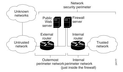
Figure 47-2 The diagram is an example of a two-perimeter network security design.
