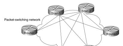
Figure 9-4 Partially meshed topology.
