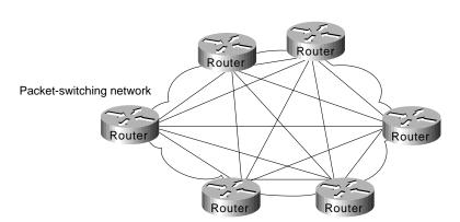
Figure 9-3 Fully meshed topology.
