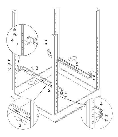
1 Slacken the M4 nuts on the left bracket. 2 Adjust the bracket to fit the rack. The ends of the bracket must be outside the rack. 3 Move the brackets so that the studs are in suitable slots and tighten the nuts. 4 Fasten the screws on both ends of the bracket. 5 Repeat for the right bracket.
