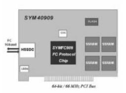
The SYM40909 implements a HSSDC type connector for copper connections up to 30 meters while the SYM40909G supports the
