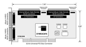
subsystems that rely on ultra differential signaling technology. For cable length and signal integrity, it also provides an expansion path for PCI slot limited servers. This adapter is popular in clustered environments where one channel is dedicated to the shared storage resource, and the other channel for that node's private storage.
