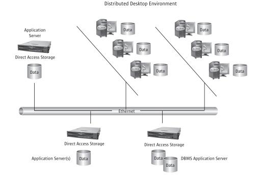
Figure 1: Distributed Computing and Storage Architecture prior to NAS Storage Consolidation
