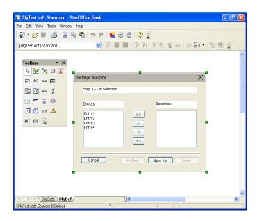
The preceding figure shows the StarOffice Basic development environment with a dialog window that contains two list boxes. You can move the data from one list to the other using the buttons between the two list boxes.
