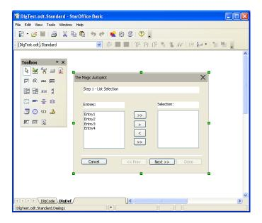
In the preceding example, you can also assign the Step value of 0 to the dividing line as well as the Cancel, Prev, Next, and Done buttons to display these elements on all pages. You can also assign the elements to an individual tab page (for example page 1).
