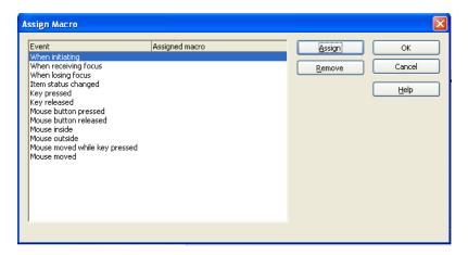
The assignment dialog lists all of the StarOffice Basic procedures. To assign a procedure to an event, select the procedure, and then click **Assign**.
