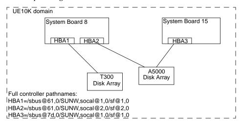
In the illustration, above, to detach or attach System Board 8, the procedure is:
