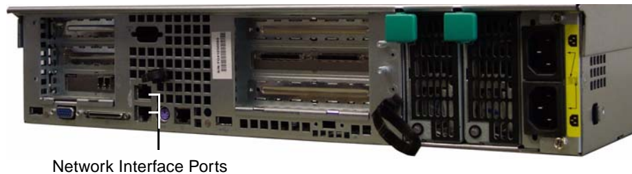
FIGURE 2-8 Connecting to Ethernet Networks
