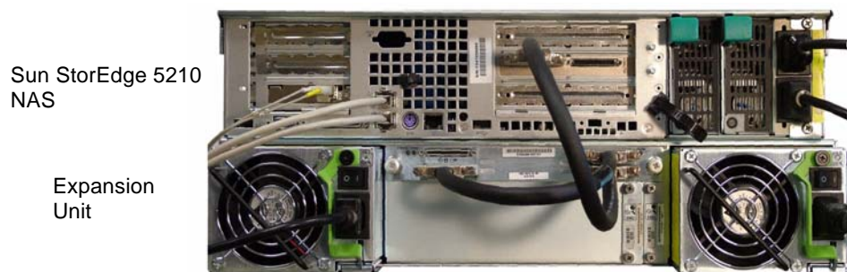
FIGURE 2-9 Connecting the Sun StorEdge 5210 NAS and a Single Expansion Unit
