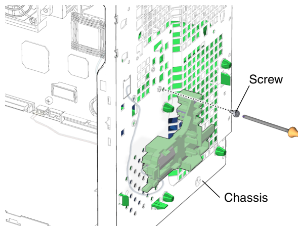
FIGURE 13-37 Installing the Screw for the Front Fan Bracket
