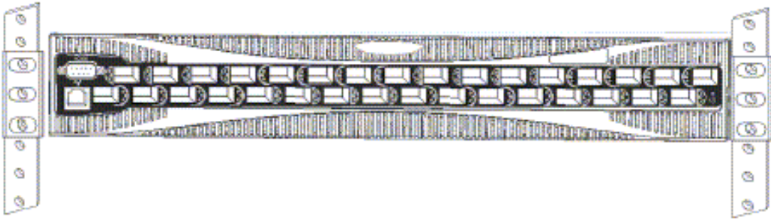
FIGURE 3-1 1.5 RU Switch Installed With the Additional 0.5 RU Above the L-Brackets
