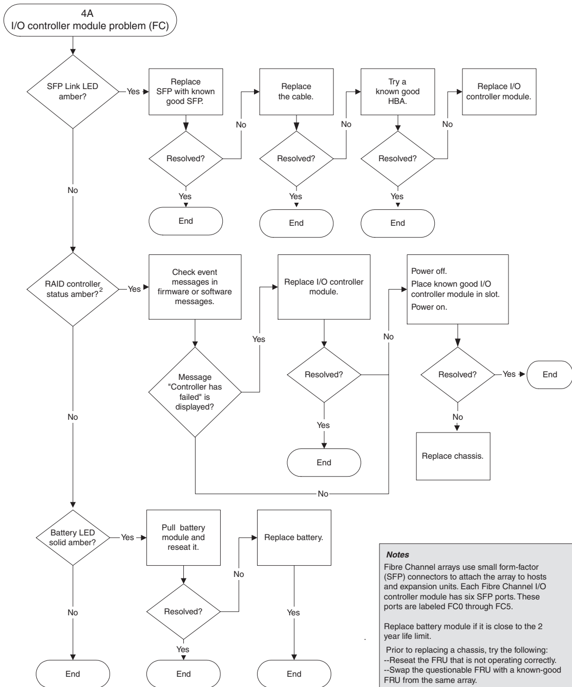
FIGURE 9-9 I/O Controller Module Flowchart
