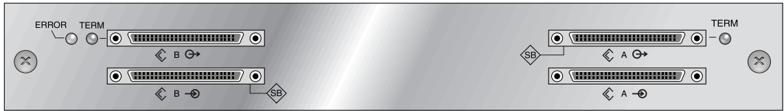
FIGURE 6-8 I/O Module for an Expansion Unit
