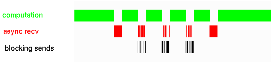
FIGURE A-4 Progress may be made on multiple messages by a single MPI call, even if that call does not explicitly reference the other messages.
