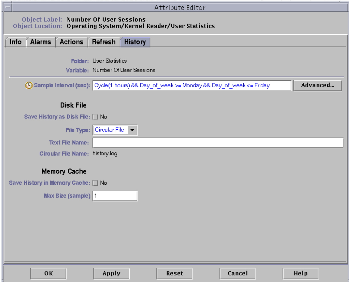
FIGURE 11-8 Updated History Attribute Editor Showing a Cycle Time of One Hour From Monday to Friday
