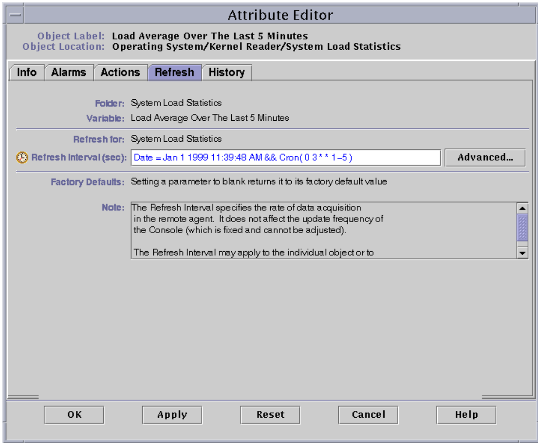
FIGURE 7-48 Refresh Interval With Starting Time of 11:39:48 AM January 1, 1999 and 3 AM Every Monday Through Friday
