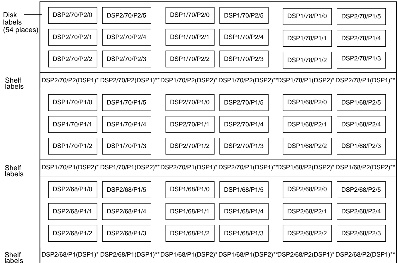
FIGURE 4-7 HDSA Disk Drive Slot Location Reference Labels, Single Drawer (Example)
