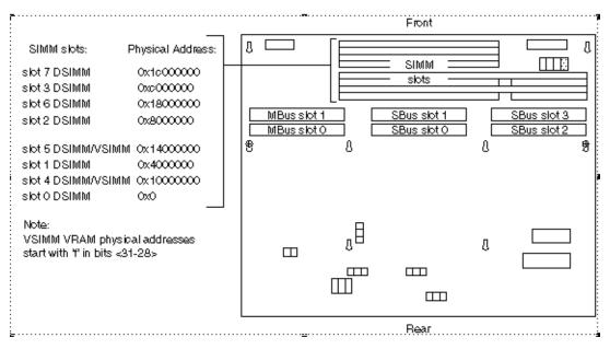
The table below illustrates the physical address map of a system configured with 16 MByte DSIMMS in all the slots
