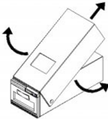
FIGURE 5-2 Removing the Cover
