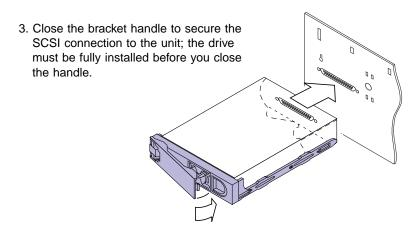
4. To remove the drive, open the bracket handle to release the SCSI connection. Pull the drive out using the handle.
