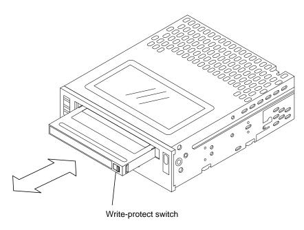
4. Push gently on the tape until the unit pulls the cartridge into the drive.
