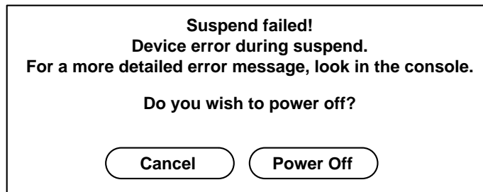
FIGURE 2-4 Suspend Failed Example
