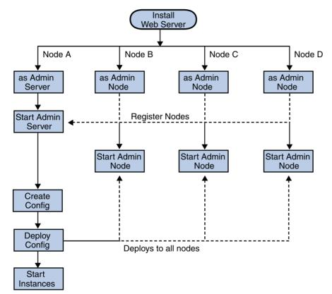
FIGURE 4-3 Flowchart illustrating the cluster set up
