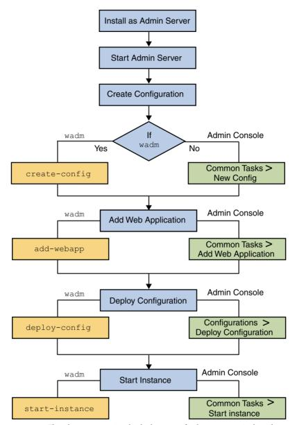
FIGURE 4-1 Flowchart representing the deployment of web server on a single node
