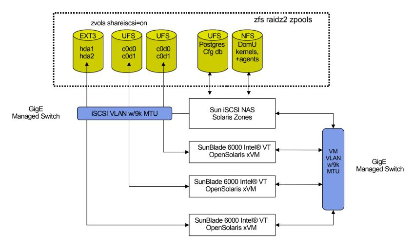
Intel e1000g NICs used for all VLANs with jumbo frames enabled & 802.3ad
