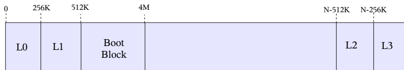
Illustration 7 Vdev label layout including boot block reserved space.
