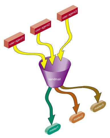
**Figure 9-2** sendmail System Structure
