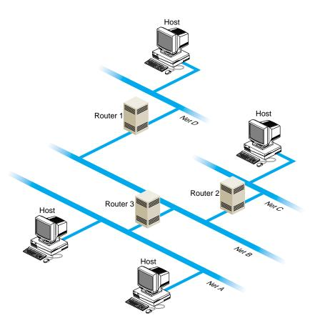
Figure 3-1 Network With Multicast Routers
