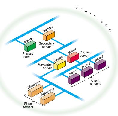
Figure 6-2 Example BIND Configuration
