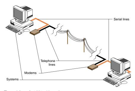
Figure 1-2 Serial Line Network
