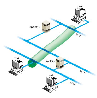
**Figure 3-2** A Tunnel Between Networks A and C
