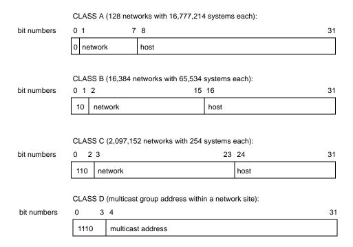
Figure 2-2 Format of Internet Protocol (IP) Version 4 Addresses
