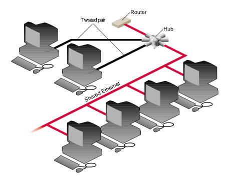
Figure 1-1 Ethernet Network Attachment
