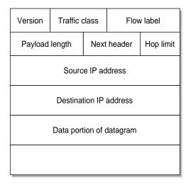
**Figure 2-5** IPv6 Header Format and Data Portion of a Datagram
