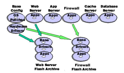
Figure 2-2: Base configurations, application profiles, and Flash archives
