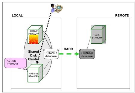
Figure 1-8 Failure of the primary node
