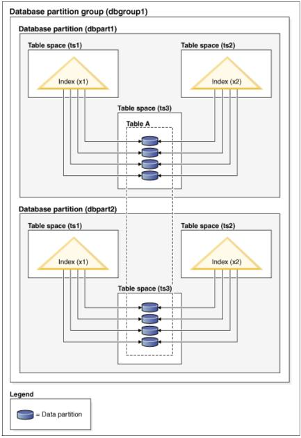
Figure 13-2 Index placement in a partitioned distributed table.
