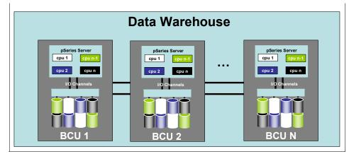
Figure 12-8 Balanced configuration unit
