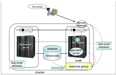
Figure 8-3 illustrates how the resource group moves during switch over.
