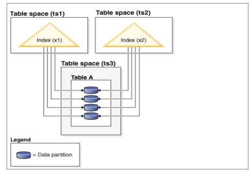
Figure 13-1 Index distribution on a partitioned table
