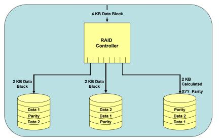
Figure 1-4 shows how a basic RAID 5 system works.
