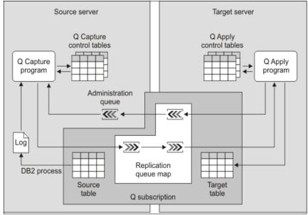
Figure 1-6 A simple configuration in Q replication
