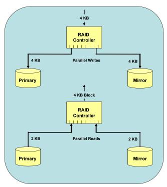
Figure 1-2 RAID 1 (disk mirroring) architecture
