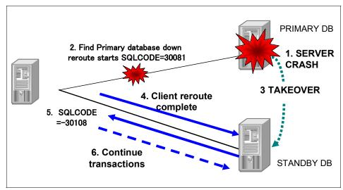
Figure 5-2 Automatic client reroute in action
