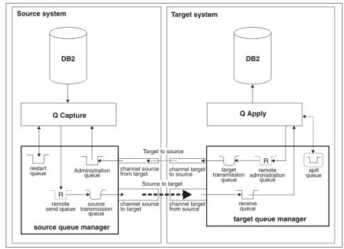
Figure 11-1 Unidirectional setup diagram
