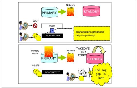
Figure 6-2 HADR behaviors when the primary cannot transfer logs to the standby
