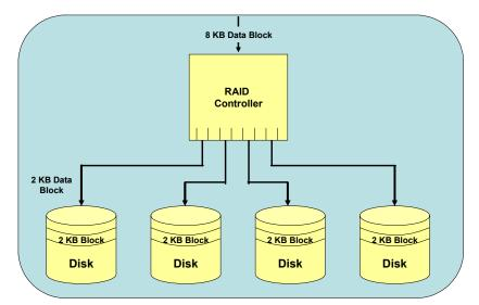
Figure 1-1 RAID 0 (disk striping) architecture
